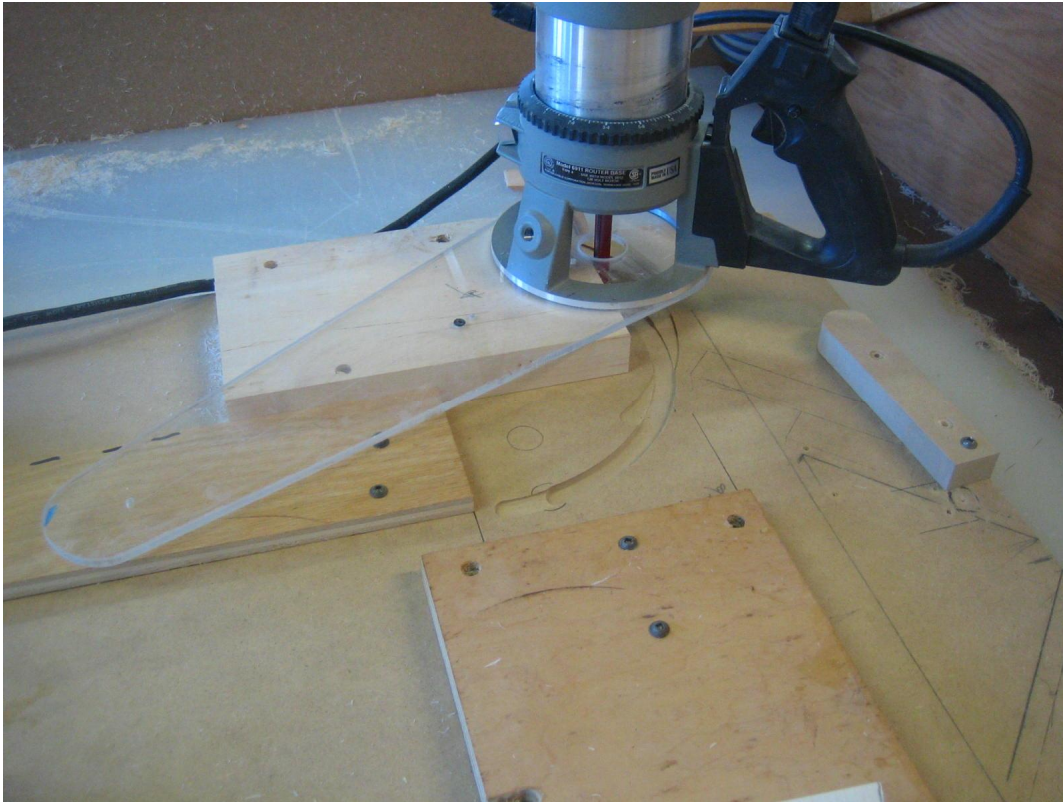
Router Fixture for cutting curved Slots
