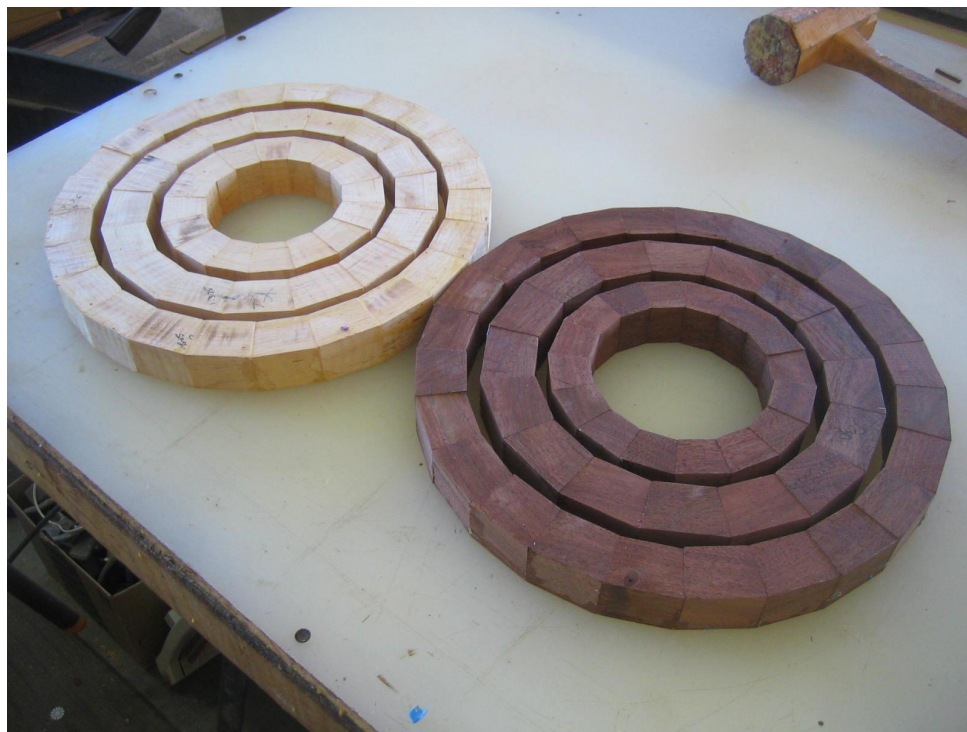
Various size rings glued up for the different divider rings. These will be cut into thinner rings on the table saw
