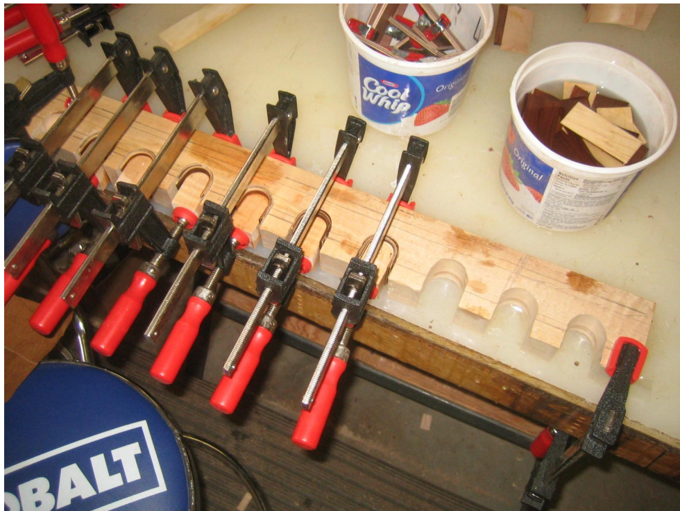
Pre-forming the 7 thin strips because the radius is too small to force the strips into the slot without breaking The strips were soaked in water for a few minutes
