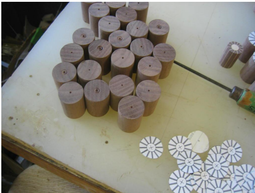
16 walnut dowel with center Marked using the Lathe for accuracy. Paper patterns printed on full sheet label paper and cut out.
