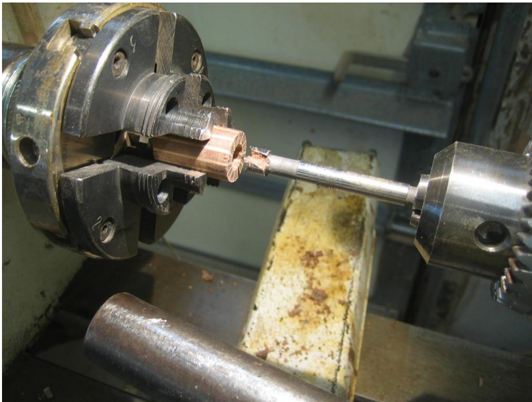
Drill out \frac{1}{4} " hole to \frac{3}{8} dia.
