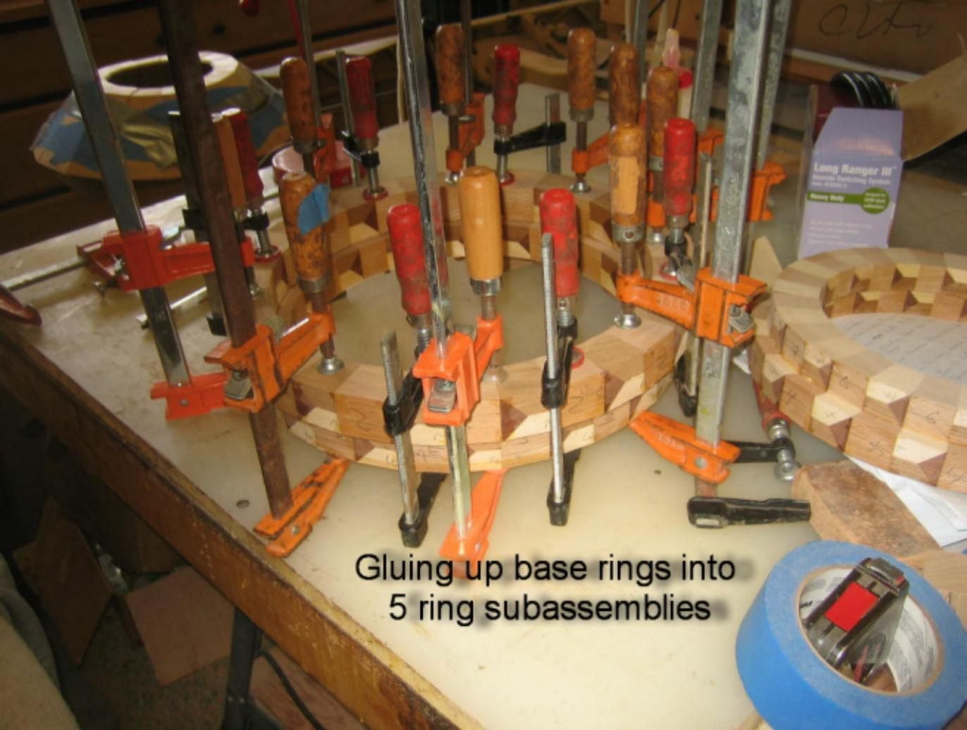
Gluing up base rings into
