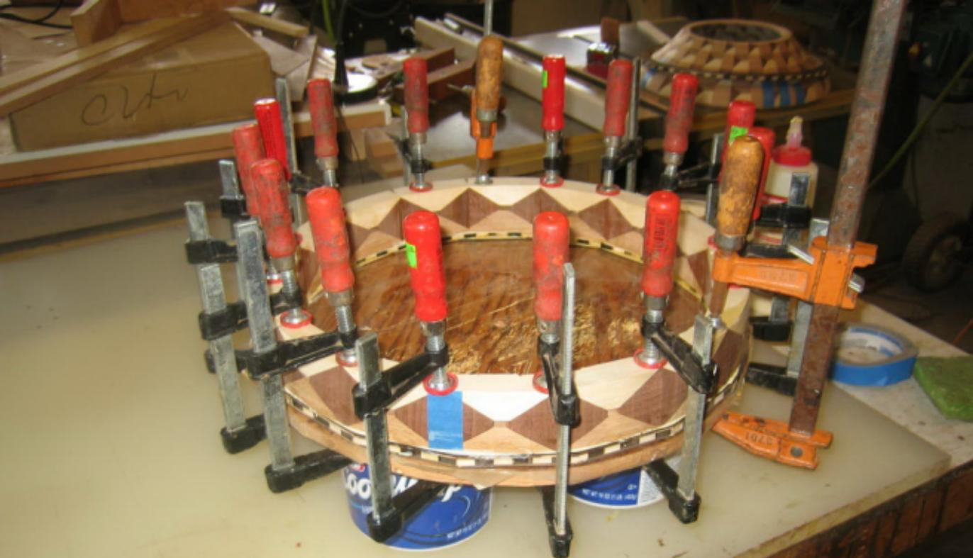
Gluing Divider Rings onto Feature ring
