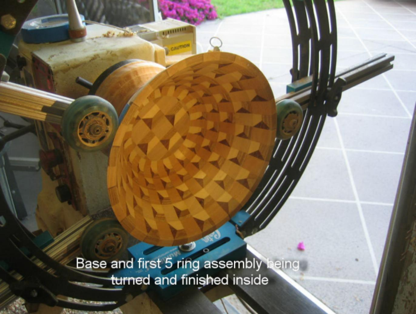
Base and first 5 ring assembly being turned and finished inside
