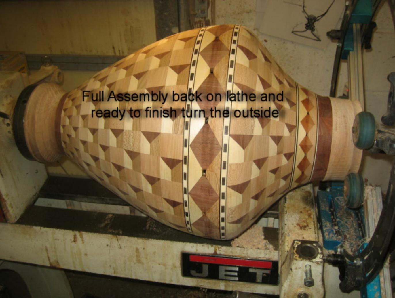
Full Assembly back on lathe and ready to finish turn the outside
