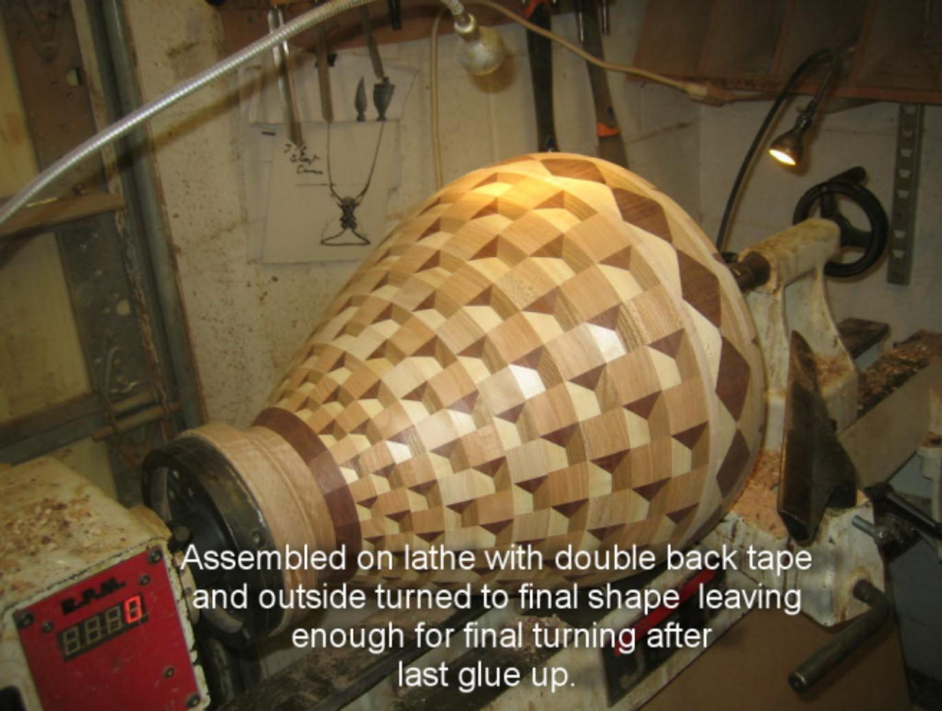
Assembled on lathe with double back tape
