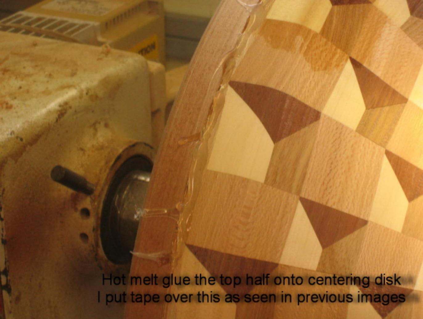
Hot melt glue the top half onto centering disk
