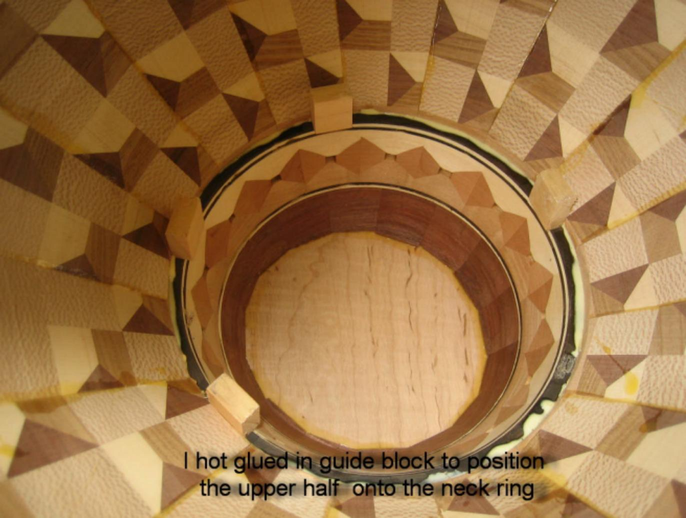
I hot glued in guide block to position
