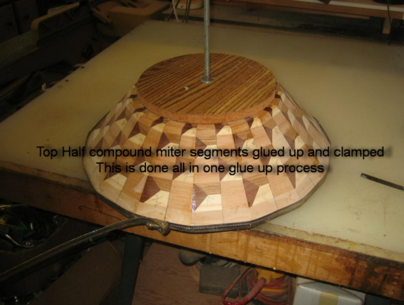
Top Half compound miter segments glued up and clamped
