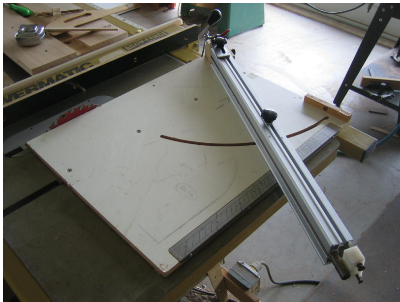
109: I make all my cuts using the Dubby cutoff sled except for the compound miter cuts.
