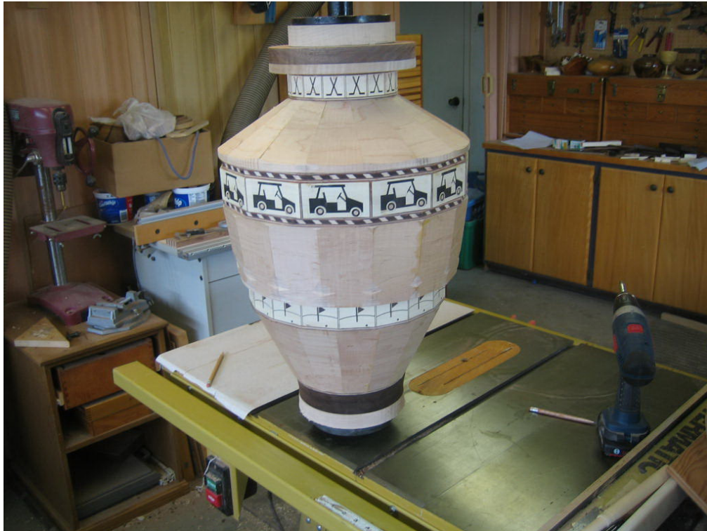
170: Outside profile turned close to final profile. Center section is still double backed taped in place
