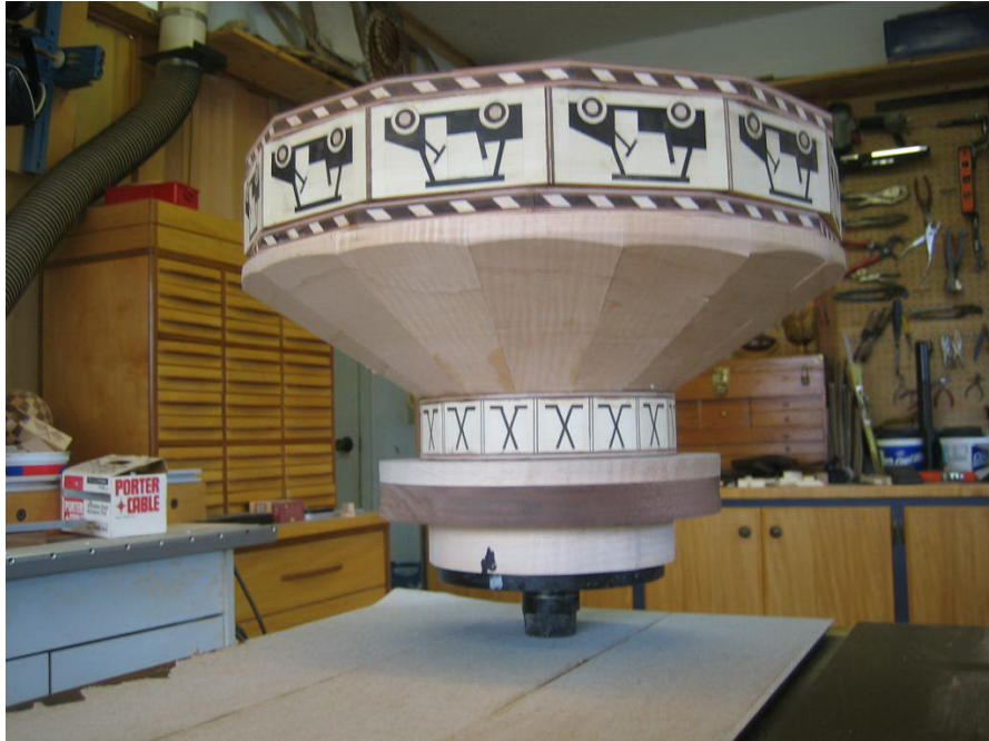
166: Bottom section in lathe ready to turn inside
