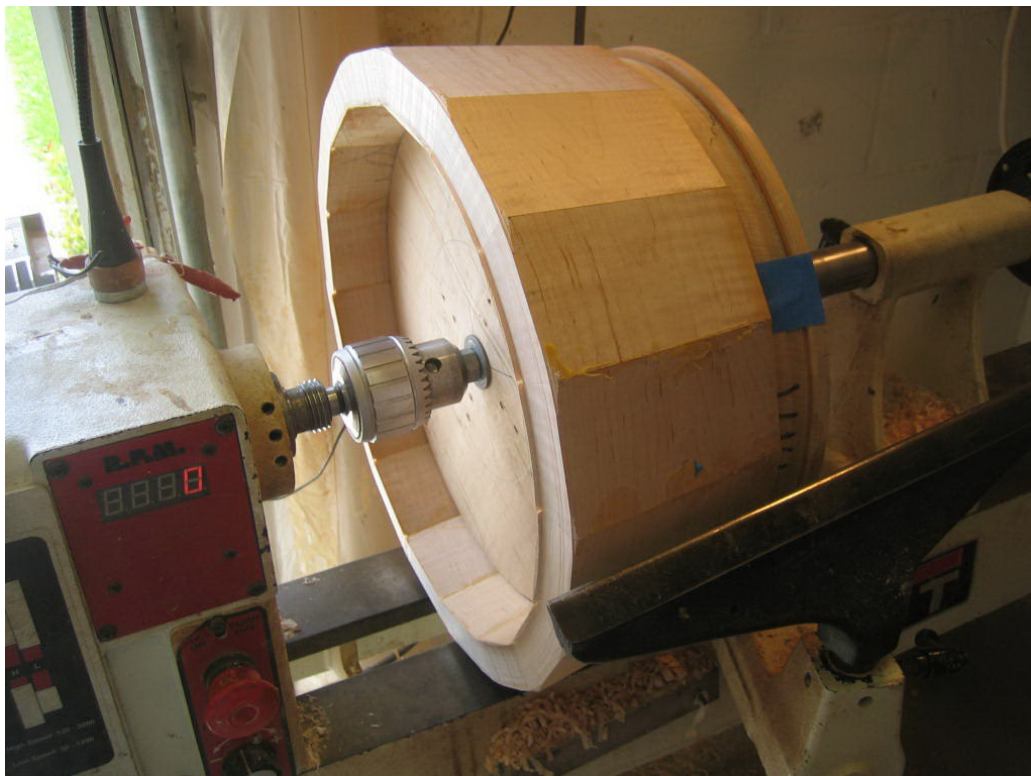
154: Ring segment setup on lathe to turn ends flat.
