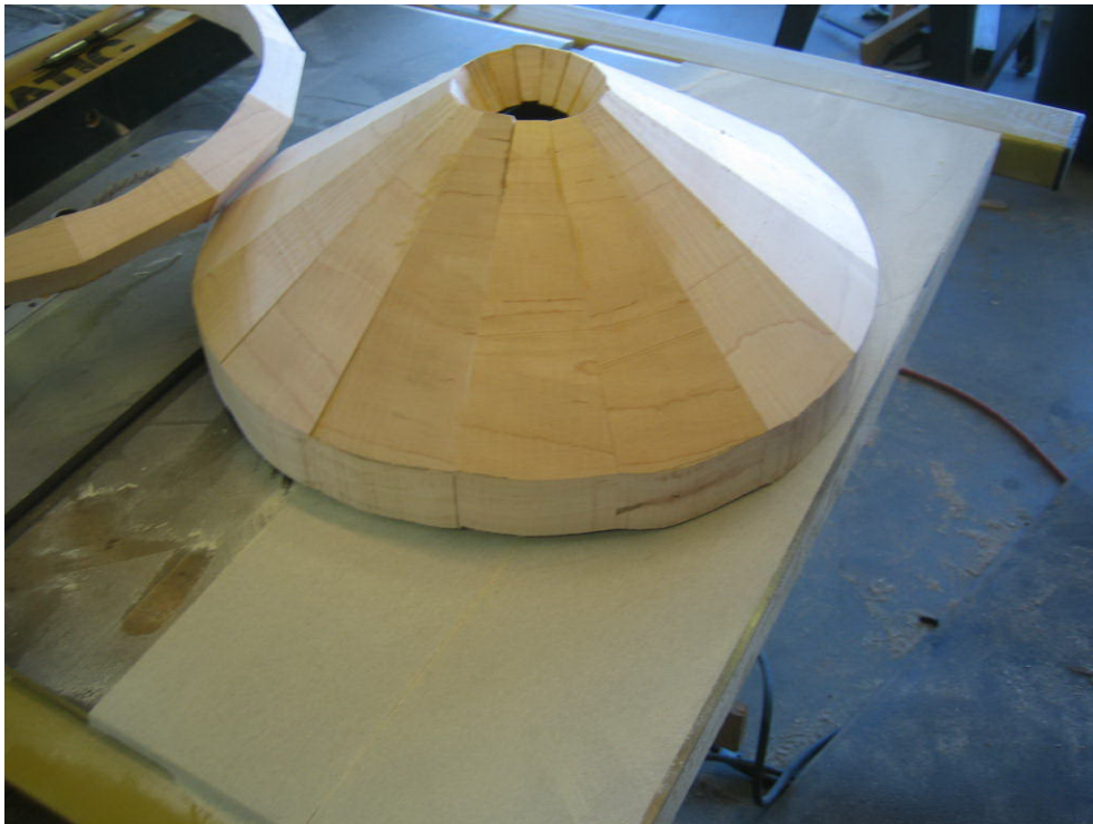
152: Top section trimmed on band saw to match feature ring.
