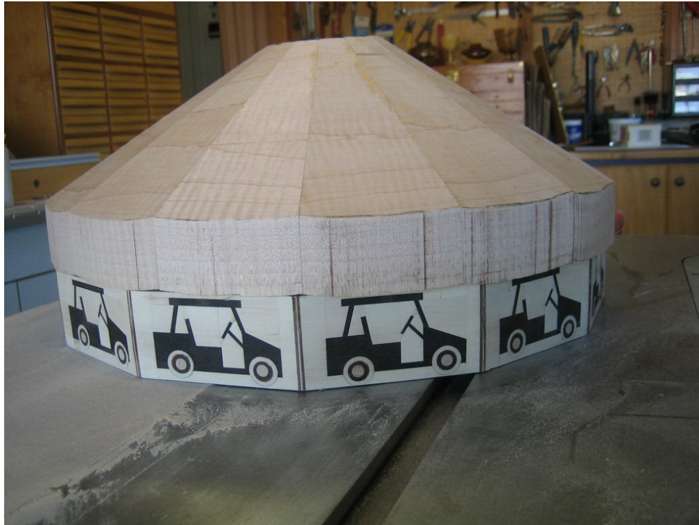
154: Ring segment setup on lathe to turn ends flat.
