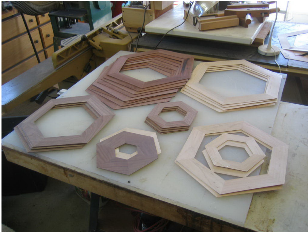
156: All spacer rings cut and sanded to the proper thickness Walnut .060 and Maple .030 I made up thick rings and sliced thin rings off them on the table saw.
