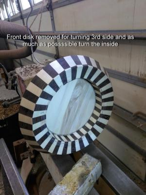
Ring reversed using Cole Jaws to finish turning and sanding. The sanding should be done complete after each surface is turned on all rings.
